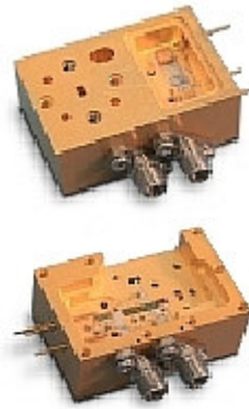
76.5 GHz FM-CW Transceiver for Vehicle Radar Application
